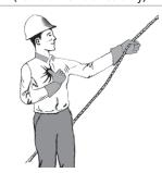
TELESCOPE OUT (TELESCOPING BOOMS)
