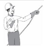
TELESCOPE IN (TELESCOPING BOOMS)
