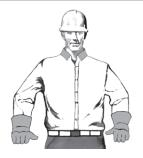
TELESCOPE IN (TELESCOPING BOOMS)
