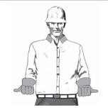
TELESCOPE OUT (TELESCOPING BOOMS)
