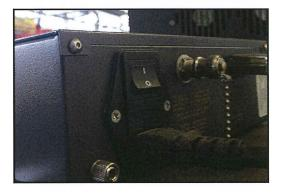
After this switch is flipped to the "on" position a green light on the front of the machine will turn on, indicating the machine is ready. Once that green light turns on, the cover can be taken off the "Laser On" button on the front and it should be pressed. This will complete the powering on of the laser.
